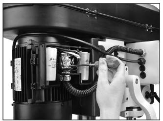
Figure 9. Changing motor jumper positions.
